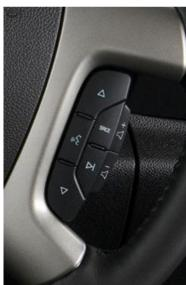
Your steering wheel buttons can be used to control your aftermarket Kenwood radio. You can assign steering wheel buttons to Kenwood radio functions. Simply program your Maestro RR module online using the Weblink updater and customize your buttons. Each steering wheel button can control up to two radio features.
