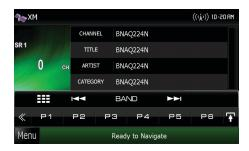
Satellite Radio must be selected during the Maestro RR online programming with the Weblink Updater. An XM subscription is required to receive XM radio services. If your tuner needs to be activated, tune to channel 0 to see your radio ESN which is required for an activation (as shown above).
