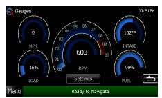
Some radios can display a needle or a bar on each gauge. If your radio supports this feature, a short press on the gauge will toggle between the needle and bar display.
