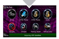
Maestro features can be accessed in the My Car submenu. If an icon is not active (grayed out) then it is not available in your vehicle or it was disabled when the Maestro module was programmed using Weblink. The options described here may not be available in your vehicle.
