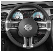
Your steering wheel buttons can be used to control your aftermarket Kenwood radio. You can assign steering wheel buttons to Kenwood radio functions. Simply program your Maestro RR module online using the Weblink updater and customize your buttons. Each steering wheel button can control up to two radio features.
