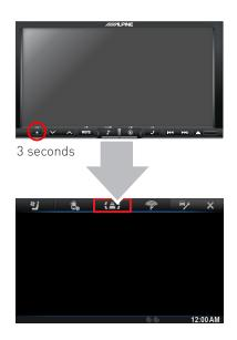
Maestro features can be accessed by pressing and holding the star button on the front of the radio for 3 seconds. If a feature is not available in your vehicle or it was disabled when the Maestro module was programmed using Weblink it will not be in the menu. The options described here may not be available in your vehicle.
